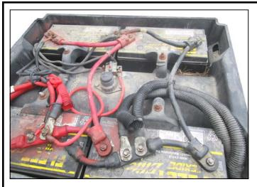
Heavy duty truck batteries are tough to handle. They're heavy, awkward . . . and when they're squeezed into a battery box, it's tough to get a grip on them for lifting . . . and lifting by the terminal posts will damage the battery . . .
